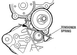
**3.** Grip the other tensioner spring projection and fit it onto the oil pump case lug as shown in the illustration. Move the timing belt tensioner in the direction shown and . temporarily tighten the bolt.
