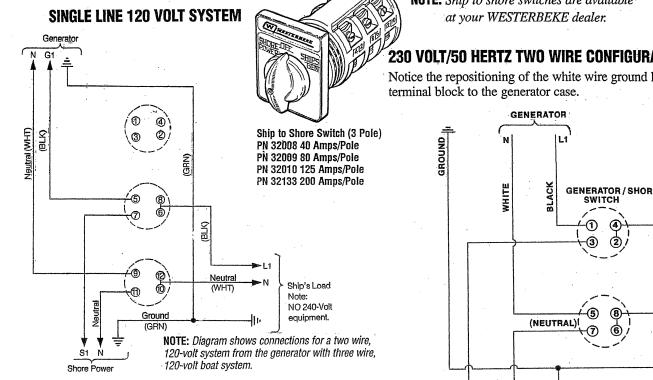
If the installer connects shore power to the vessel's AC circuit, this must be done by means of the Shore Power Transfer Switch. Set the transfer switch shown in the diagrams to the OFF position. This switch prevents simultaneous connection of shore power to generator output.
