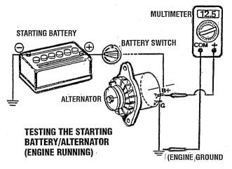
8. Start the engine again. Check the voltage between the alternator output and ground.
