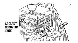
**NOTE:** Periodically check the condition of the manifold pressure cap, its rubber seals and the vacuum return valve. Ensure the passage from the filler neck to the recovery tank connection is kept clear.
