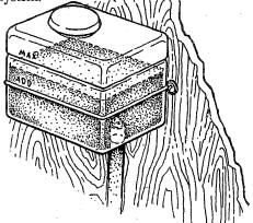
**NOTE:** This tank, with its short run of plastic hose, is best located at or above the level of the engine's exhaust manifold.
