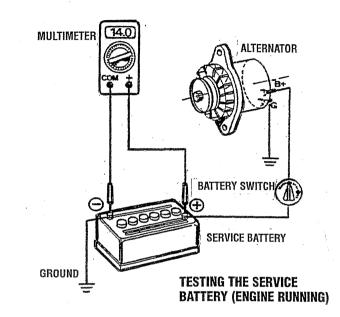
**CAUTION:** To avoid damaging the alternator diodes, do not use a high voltage tester (i.e. a megger) when performing tests on the alternator charging circuit.
