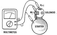
NOTE: Disconnect the wire from terminal M.
