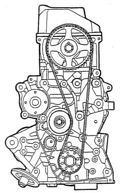
5. Turn the crankshaft twice in the normal rotating direction (clockwise) and check that the timing marks are correctly aligned.
