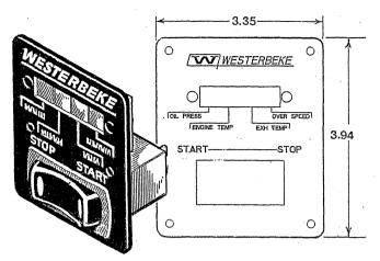
Refer to page 7 (*CONTROL PANEL START/STOP PROCEDURE*) for additional instructions and warnings. **REMOTE PANEL HARNESS:** 15' Pn 049210
