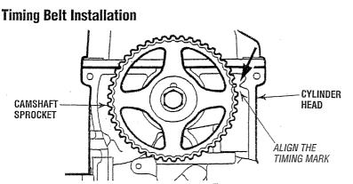
1. Align the camshaft timing mark with the timing mark on the cylinder head.
