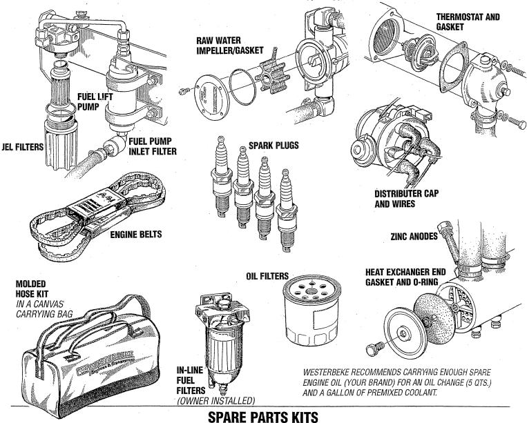
WESTERBEKE also offers two Spare Parts Kits, each packaged in a rugged, rust free toolbox. **KIT A** includes the basic spares. **KIT B** is for more extensive off-shore cruising.
